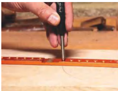
▲ A series of holes allows bowl blanks to be marked up for cutting
